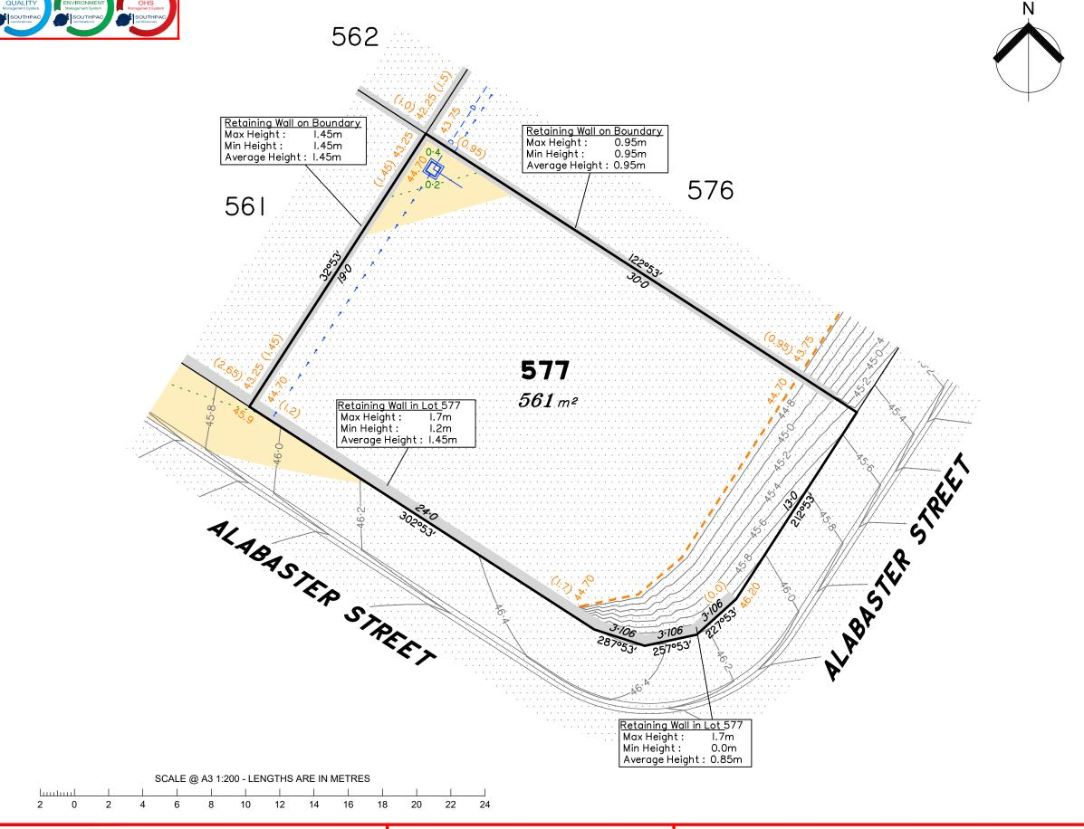
LEGEND Area of Cut Area of Fill Finished Surface Contours - - Depth of Fill Contours Retaining Wall (1.0)(Visible height shown on lower side of wall) Proposed Earthworks Pad 43.25 Finished Design Surface Level Future Lot Boundary Stormwater Drainage Line Stormwater Drainage Swale Line Stormwater Field Inlet
