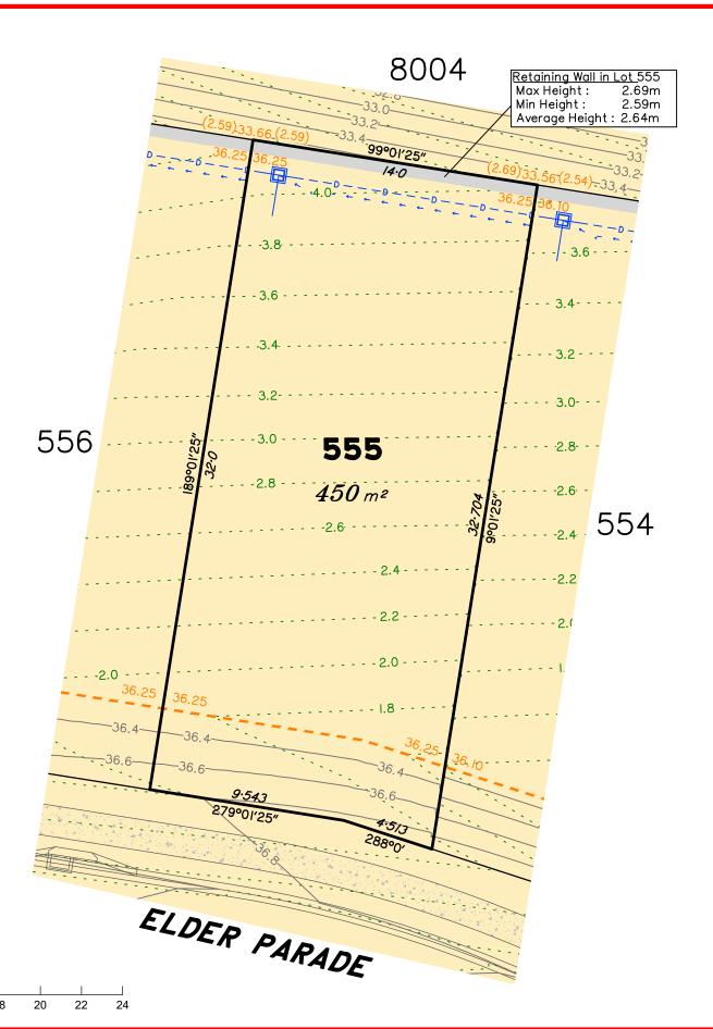
LEGEND Area of Cut Area of Fill **Finished Surface Contours** - - - Depth of Fill Contours Retaining Wall (Visible height shown on lower side of wall) Proposed Earthworks Pad 43.25 Finished Design Surface Level Future Lot Boundary Stormwater Drainage Line Stormwater Drainage Swale Line Stormwater Field Inlet
