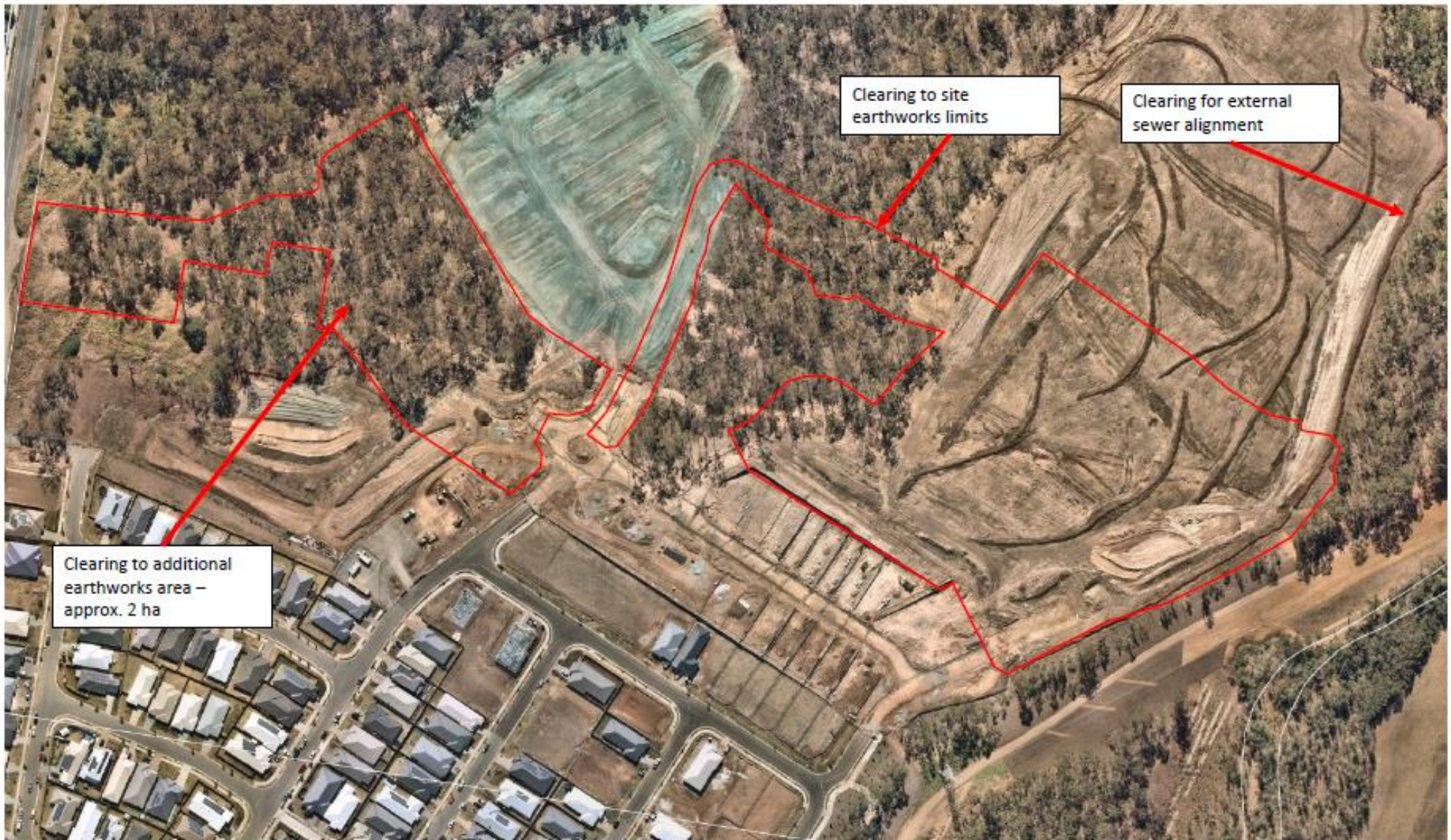
Figure 1- Extent of clearing
