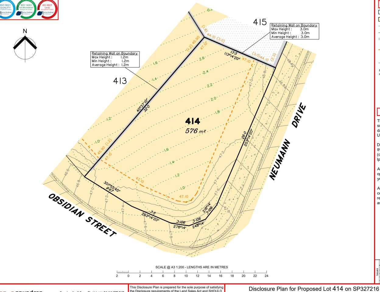
Area of Fill **Finished Surface Contours** - - Depth of Fill Contours Retaining Wall (Visible height shown on lower side of wall) Proposed Earthworks Pad 38.78 Finished Design Surface Level — Future Lot Boundary Not all items in this legend may be relevant to the lot shown on this plan. NOTES This plan has been prepared from preliminary survey plan (SP327216) and engineering data provided on the 27/04/2021 by Peak Urban Pty Ltd. Development approval has been received for
