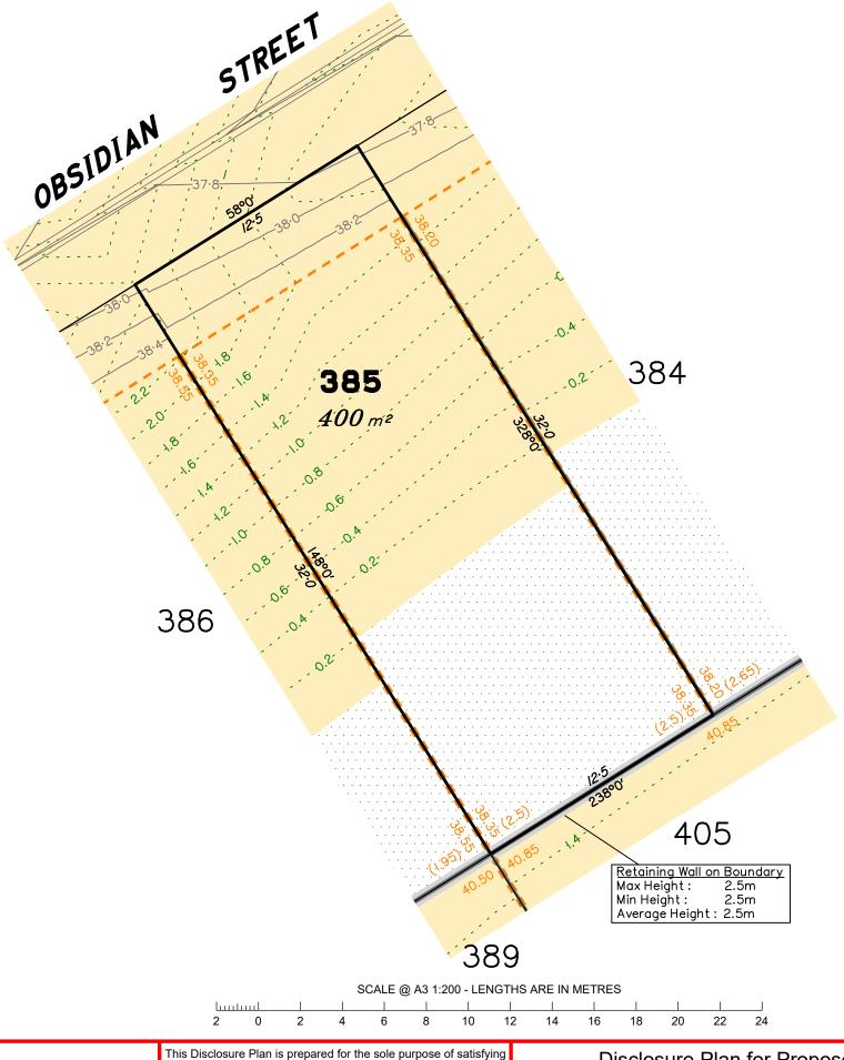
Area of Cut Area of Fill **Finished Surface Contours** - - - - Depth of Fill Contours Retaining Wall (Visible height shown on lower side of wall) Proposed Earthworks Pad 38.78 Finished Design Surface Level — Future Lot Boundary Not all items in this legend may be relevant to the lot shown on this plan.
