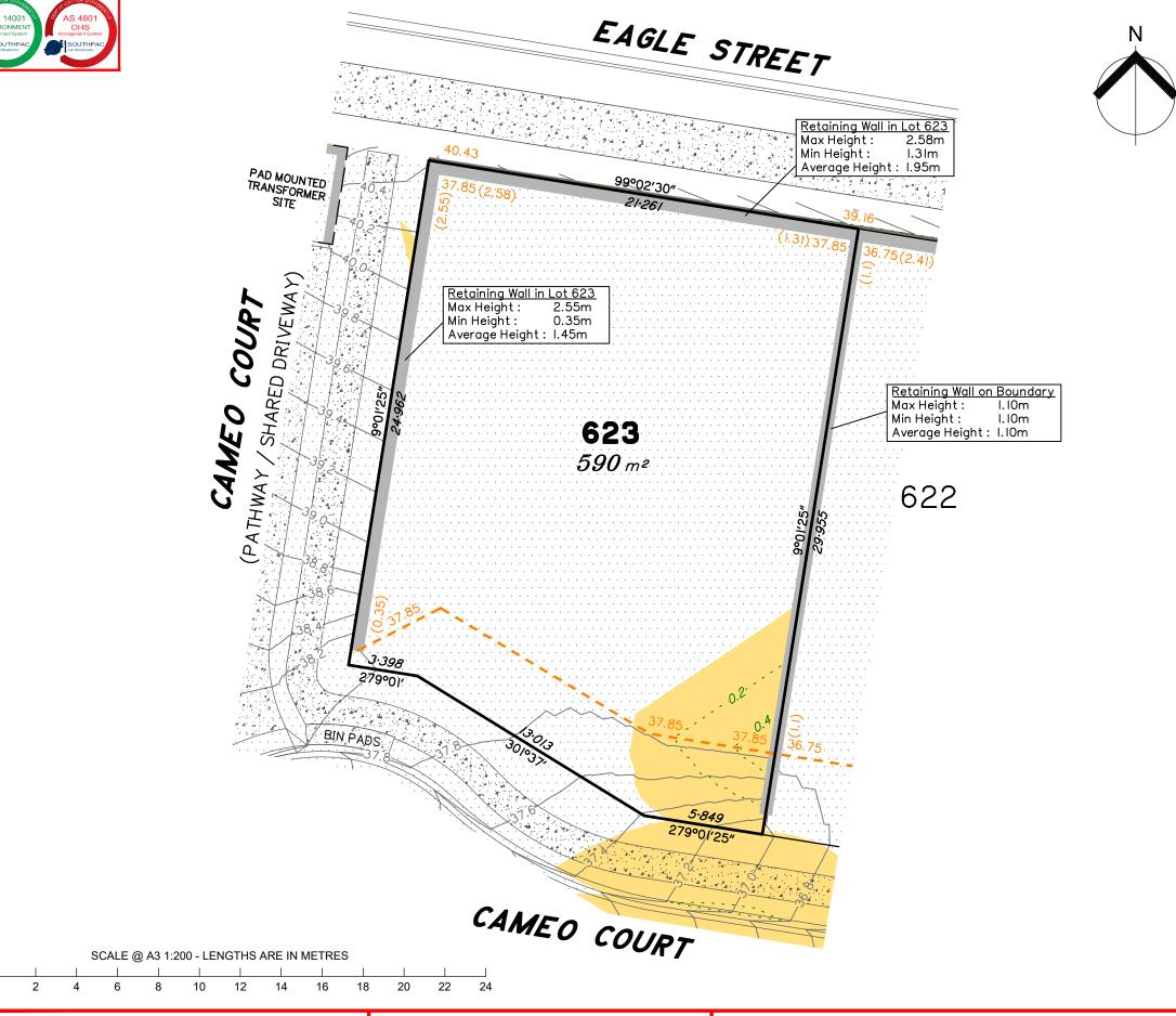
LEGEND Area of Cut Area of Fill Finished Surface Contours Depth of Fill Contours Retaining Wall (1.0)(Visible height shown on lower side of wall) Proposed Earthworks Pad Finished Design Surface Level Future Lot Boundary Sewer Line / Manhole Drainage Line / Pit
